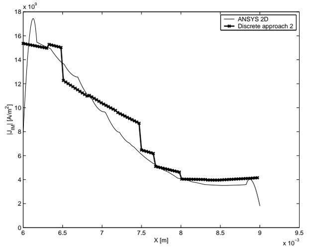
Figure 8. The absolute values of the imaginary part of current density along  $l_2$ .
