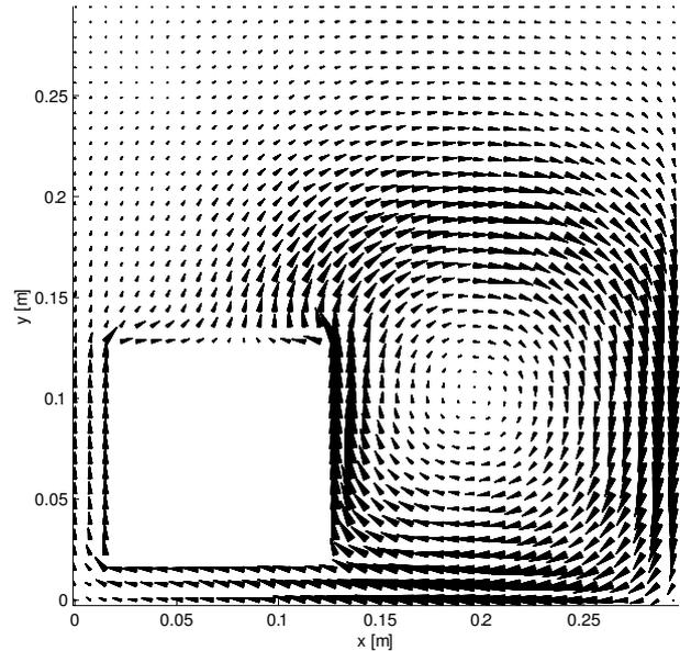
Figure 10: The induced current in the plate.
