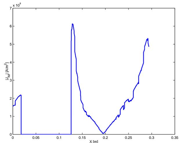
Figure 12. The absolute value of the imaginary part of induced current density along the line (TEAM problem 7 geometry).
