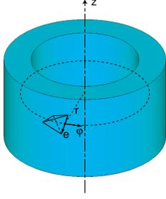
Figure 1. Geometry of source region  $D_s$  in the case of a circular coil.
