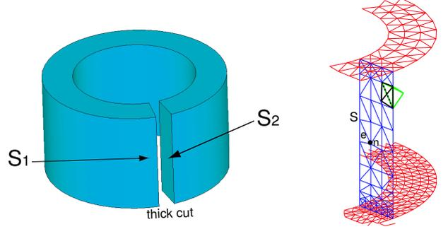
Figure 2. On the left the coil with the air cut are shown, together with the pair of surfaces  $S_1, S_2$  between the thick cut and the conductor. On the right nodes like  $n$  and edges like  $e$  laying on  $S$  have duplicated labels.
