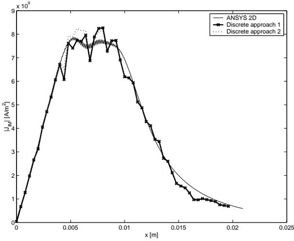
Figure 6. The absolute values of the imaginary part of current density along  $l_1$ .
