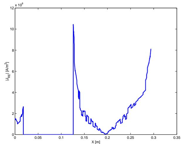
Figure 11. The absolute value of the real part of induced current density along the line (TEAM problem 7 geometry).
